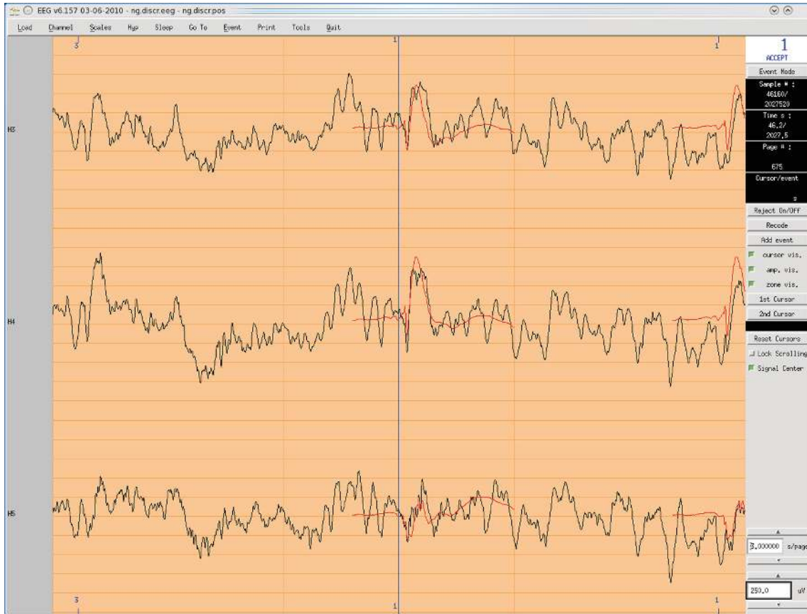
FIGURE 1: EEG visualization tool for continuous data (.eeg file), with an example of intracranial auditory EEG signals. X-axis: time, Y-axis: signal amplitude, one row per channel. Events are displayed above and below the continuous EEG signals, and the averaged event-related response is superimposed in red. Various plotting tools and online analysis functions are available through the menus (top and right of the window).
