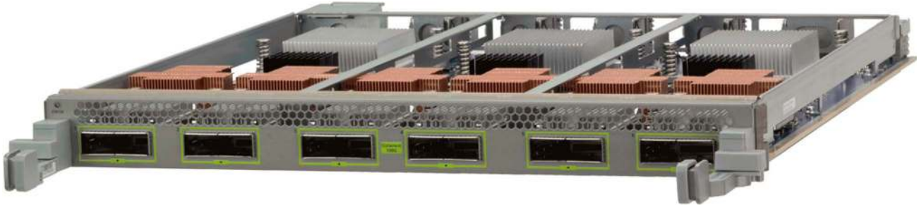
Fig. 10. Arista 7500E-series layer 2/3 six-port coherent DWDM linecard.
