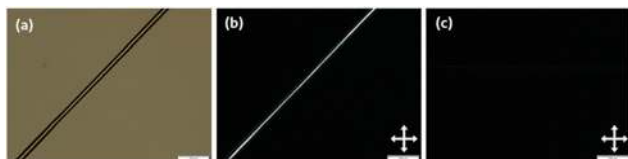
Fig. 4 A PI fibre spun from a solution of 14% w/w PI in n -hexane, slightly stretched and freely-hanging without a supporting substrate. Scale bars indicate 100 \mu\text{m} . (a) A fibre viewed with linearly polarised light without an analyser. (b) The same fibre in (a) viewed between crossed polarisers; arrows indicate the direction of the linear polarisers. (c) As (b), but upon 45° clockwise rotation to align the fibre along the direction of the polariser, showing a complete extinction of the birefringence.
