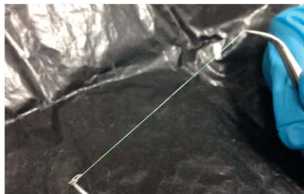
Fig. 8 A long (~20 cm) sample of a PI fibre filled with a mixture of 25% w/w ZLI-3786 in RO-TN 615, viewed under ambient room lighting.
