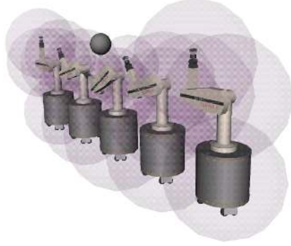
Figure 1: Elastic tunnel: The union of the local free space, shown as transparent spheres, of five configurations along the elastic strip make up the elastic tunnel. A spherical obstacle has modified the trajectory and the associated representation of free space.
