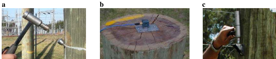
Fig. 18 (a) Modally tuned impact hammer (PCB HP 086C05) and steel bolt, (b) piezoelectric accelerometer (PCB 356A08) and mounted steel plate, and (c) impact bracket.
