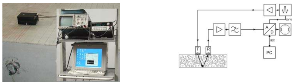
Fig. 8 Excitation of transmitting/receiving (T/R) transducer with arbitrary function generator, power amplifier (not imaged) and oscilloscope ( left ). Principle sketch for working with arbitrary pulses and data processing ( right ).
