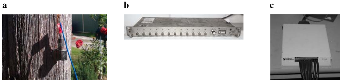
Fig. 19 (a) Piezoelectric accelerometer (PCB 352C34), (b) Multi-channel signal conditioner (PCB 483B03), and (c) data acquisition system (NI PCI-6133).
