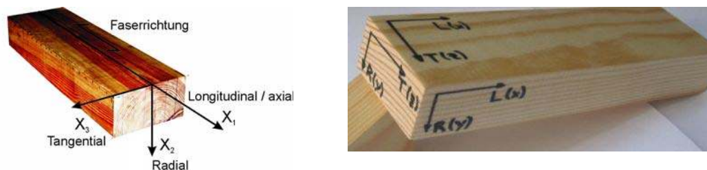
Fig. 1 Timber beam (dimension: Naming of axes of symmetry in timber: Longitudinal (L~ X_1 ), Radial (R~ X_2 ), Tangential (T~ X_3 ), image cited from [3] (left). Small specimen as used for specimens of glue laminated timber with quasi homogeneous anisotropic conditions (negligible curvature of annual rings) (right).
