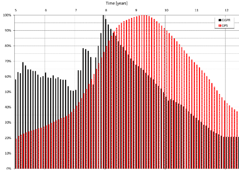
Figure 1. Monthly data for platform B: gas production rate (GGPR) versus GPS rate filtered from seasonal component.
