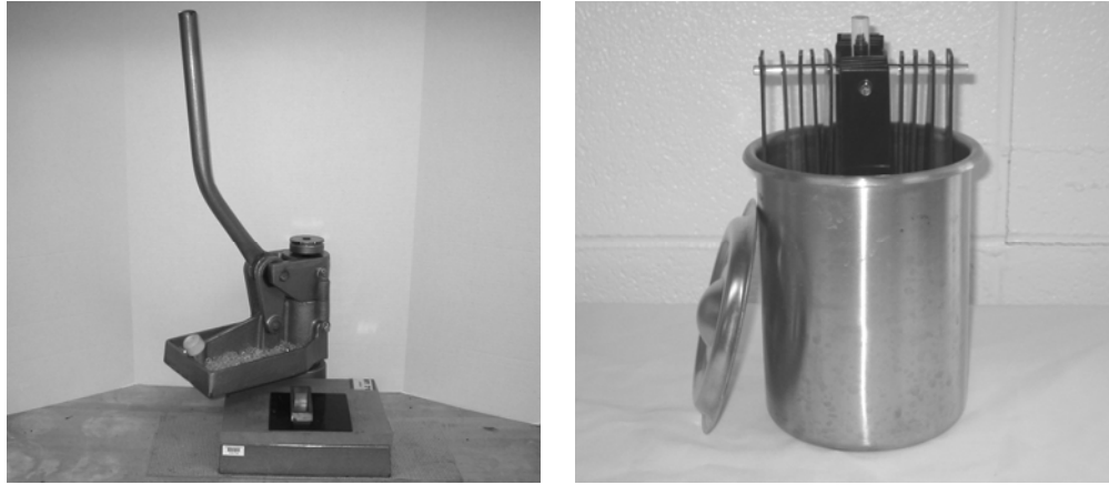
Figure 2.4 Rubber slab, die and press (left), samples cut and loaded in stainless steel cylinder (right)
