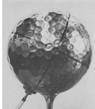
Figure 5: Nearly perfect electroformed spherical shell under external pressure [41] - in this picture, the post-buckling pattern is "artificially" stabilized because there is a solid mandrel inside the shell (adapted from [11])
