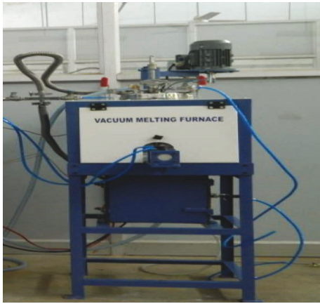
FIGURE 1: Pictorial view of magnesium stir casting setup.
