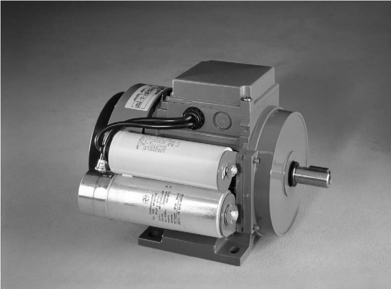
Plate 6.1 Single-phase capacitor-run induction motor. Output power range is typically from about 70 W to 2.2 kW, with pole-numbers from 2 to 8. (Photo courtesy of ABB)
