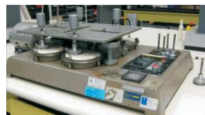
Figure 4. Abrasion resistance apparatus
