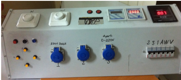
Figure 3. Isolated and regulated power supply circuit
