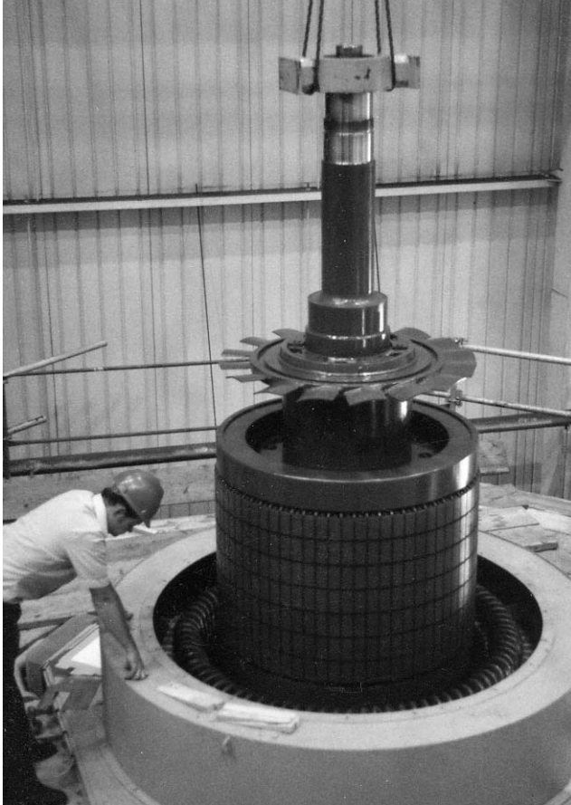
Figure 1.1. Photograph of a SCI rotor being lowered into the squirrel cage induction motor stator.
