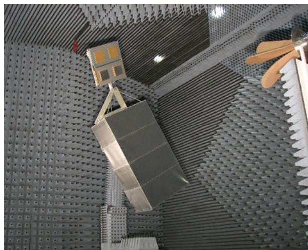
Fig. 5 Measurement of the feed array on top of the BIOMASS satellite model (Conf. 3) at the DTU-ESA Facility
