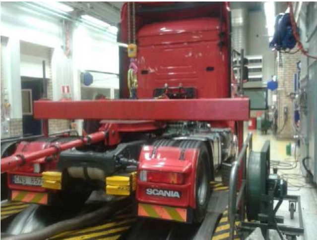
Figure 20. Truck equipped with the TEGs during the tests in the dyno-cell.
