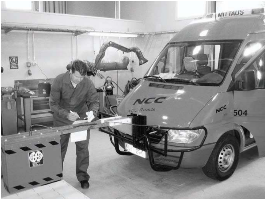
Fig. 24. GPR system testing with a 1.0 GHz horn antenna at the Rovaniemi Polytechnic laboratory which has been authorized to perform these tests in Finland. All of the GPR systems used in asphalt quality control measurements in Finland must pass these tests annually (photo Manu Marttinen).
