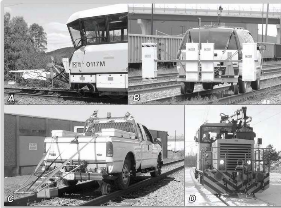
Fig. 45. Different GPR antennas used in railway surveys. Photo (A) presents a Swedish Mala ground coupled antenna (photo by Mala Geoscience), photo (B) presents a multichannel GSSI air coupled system (from Olhoeft et al. 2004), photo (C) presents a GSSI 400 MHz ground coupled antenna and photo (D) presents Radar Team Sweden 350 MHz 1.2 GHz Sub-Echo HBD antennas (photo Mika Silvast).
