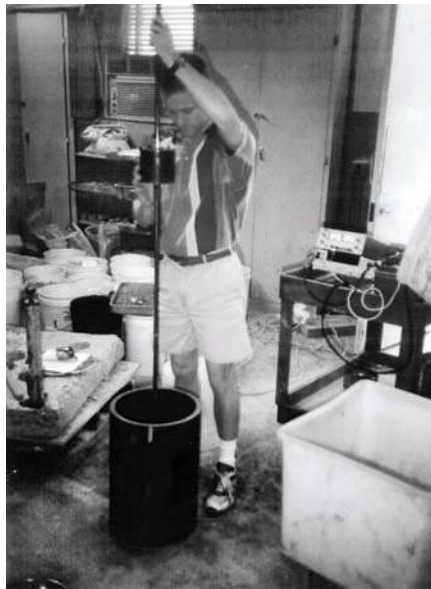
Fig. 4. DCP testing at the Texas Transportation Institute research laboratory. The aggregates were compacted at different moisture levels in the bucket. Dielectric value and electrical conductivity was measured from the DCP hole using a Percometer tube probe.
