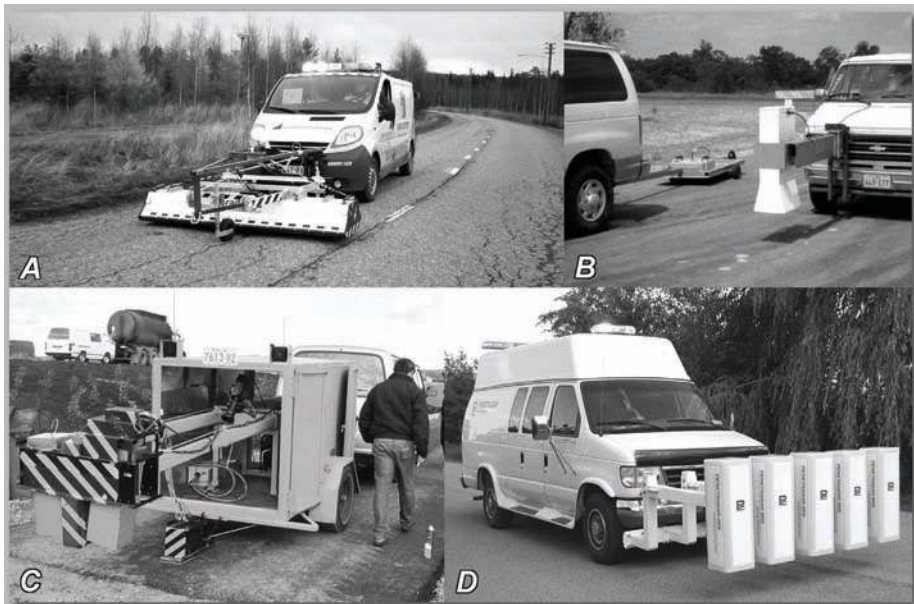
Fig. 23. Different GPR systems and antenna configurations used in road surveys. Photo (A) presents a multichannel stepped frequency radar by 3-D Radar from Norway, photo (B) presents a 100 MHz GSSI ground coupled antenna and a 1.0 GHz Pulse Radar antenna used by the Texas Transportation Institute (TTI), photo (C) presents a Canadian Road Radar system, that has a horn antenna system and a multichannel ground coupled antenna array (see Davis et al. 1994), and photo (D) presents a multichannel air coupled horn antenna system by Penetradar (photo Penetradar).
