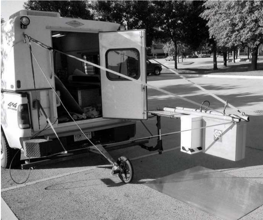
Fig. 43. Dual polarization configuration of horn antennas for high-speed, high-resolution bridge deck surveys (photo Francisco Romero).
