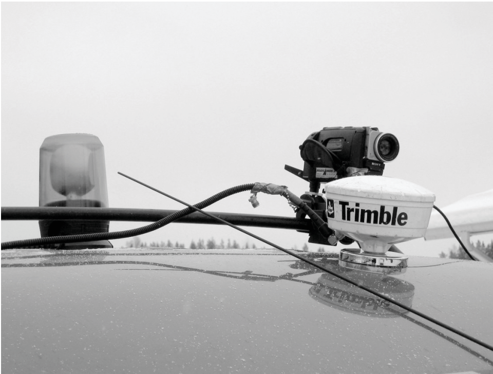
Fig. 26. A GPS and video system installed on the roof of a GPR car (photo Saara Aho).
