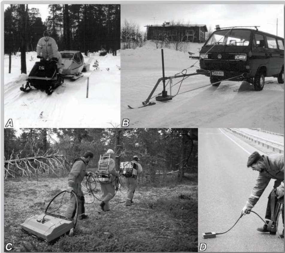
Fig. 1. GPR surveys in mid and late 1980's by the Finnish National Road Administration, Lapland Road Region projects. Photo A is a site investigation for a new road surveys line on road 91 Ivalo-Rajajooseppi using Geo-Work Oy's GPR systems with an 80 MHz antenna. Photo B presents tests for measuring ice thickness of a winter road crossing the Kemijoki river in Sierilä, near Rovaniemi. Photo C presents the use of a GSSI SIR-8 system with a 100 MHz antenna for sand and gravel prospecting in North-Eastern Lapland and photo D presents bridge deck cross section data collection using a 1.5 GHz antenna on Kulpinputaa bridge on HW4 near Rovaniemi.
