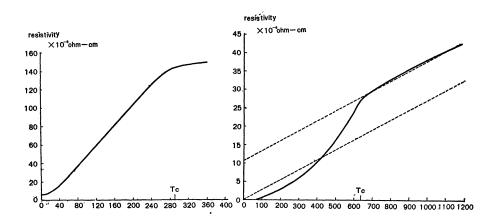
part is that when the temperature is higher the Curie temperature  $T_c$ , the resistance is almost constant, and when the temperature is lower than  $T_c$ , the resistance decreases to become zero at absolute temperature zero.
