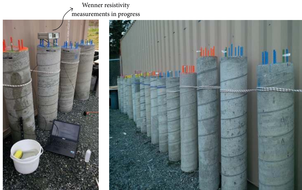
FIGURE 13: Instrumented circular hollow columns being studied by authors to establish the relationship between electrical resistivity and durability characteristics.
