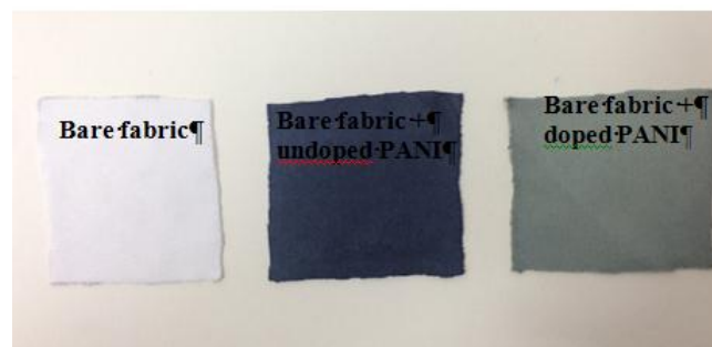
Fig.1: Visual assessment of the immersed fabric into the undoped (blue color) and doped PANI (green color).
