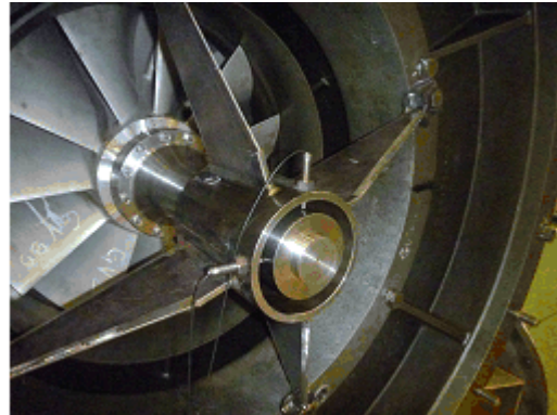
FIGURE 2. DUMMY ROTOR VIBRATION MEASUREMENT TEST
