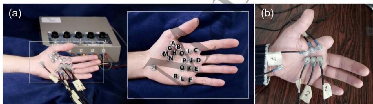
Figure 1 Experimental setup. (a) Electro-tactile stimulator connected to a subset of stimulation electrodes. The inset shows the detailed placement of the stimulation electrodes on the palm of one non-amputee participant. (b) Representative placement of the electrodes on one amputee participant.
