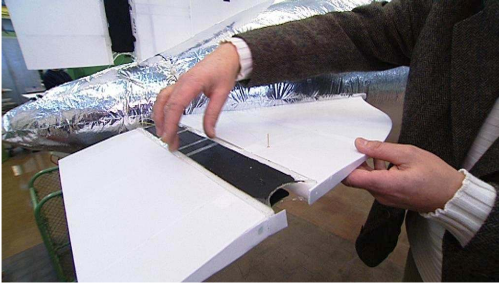
Fig. 7. Active hinge placed between the rudder (left) and the control surface (right) of the horizontal stabilizer.
