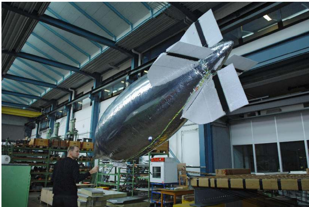
Fig. 9. Picture of the EAP blimp, with the second version of the cross tail: active hinges between the control surfaces and the rudders.
