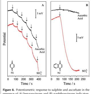
presence of (A) benzoquinone and (B) naphthoquinone indicators. Recorded at a carbon-loaded polyethylene-film electrode in pH 7 buffer.
