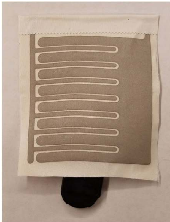
Figure 1. Photograph of an in-house developed prototype of a printed electroceutical dressing (PED) which has Ag/AgCl electrodes printed on silk and powered via to a 6 V battery 13 .
