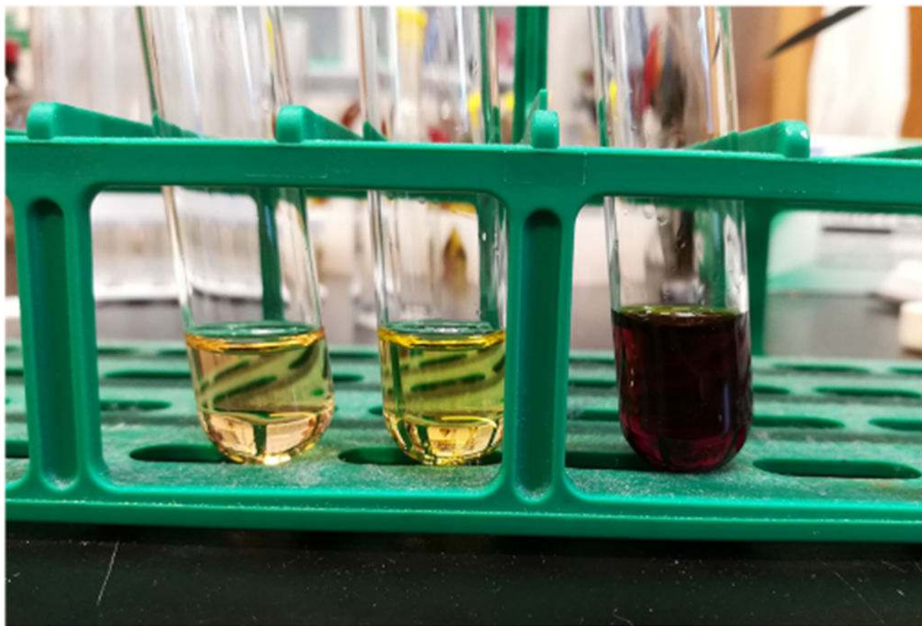
Figure 4. Color of the MeCN solution of TEMPO–N 3 adduct (right) in comparison to TEMPO • (left) and TEMPO + (center).
