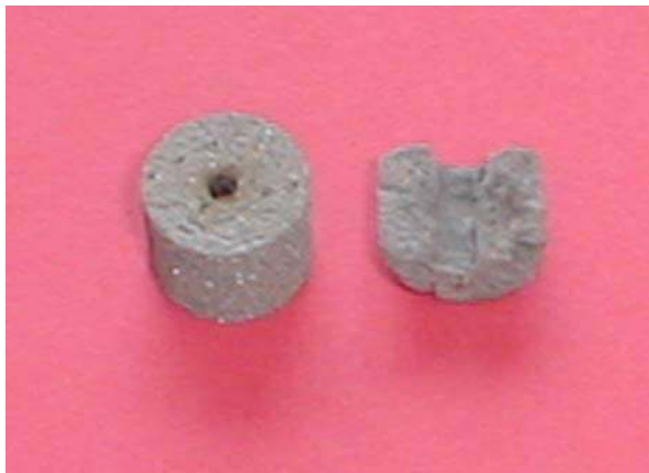
Fig. 6—Photograph of the foam before (left) and a section of the same sample after (right) deoxidation. The deoxidized sample is almost free from carbon contamination. Electrolyte: fresh (and pre-electrolyzed) CaCl 2 (Fluka, granular variety); electrolyte temperature: 950 °C; applied voltage: 2.8 V; duration of polarization: 25 h; and residual oxygen content: 0.1702 pct.
