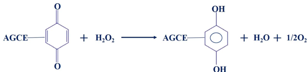
Scheme 2. Schematic representation of AGCE for the electro-catalytic reduction of \text{H}_2\text{O}_2 .
