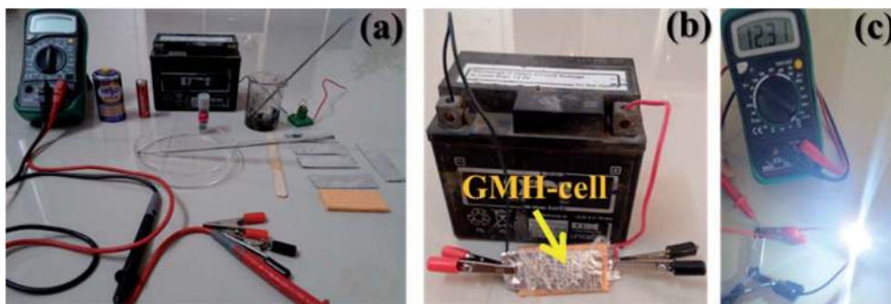
Fig. 10 Laboratory scale demonstration of GMH electrode demonstrating LED illumination. (a) Apparatus with the substrate, digital multimeter, 12.4 V commercial automobile battery, active electrode material, carbon powder, PVDF, etc., (b) charging of the blend-cell with a battery, (c) LED illumination after charging, indicating the voltage attained by the fully sealed fabricated blend electrode assembly.
