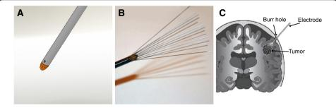
**Figure 5 Retractable brain electrodes. A)** Rendering of the electrode in fully retracted state. **B)** Electrode in fully extended state. Recommended voltage is 1000 V for the fully extended electrodes. **C)** Diagram of the insertion into brain [105].
