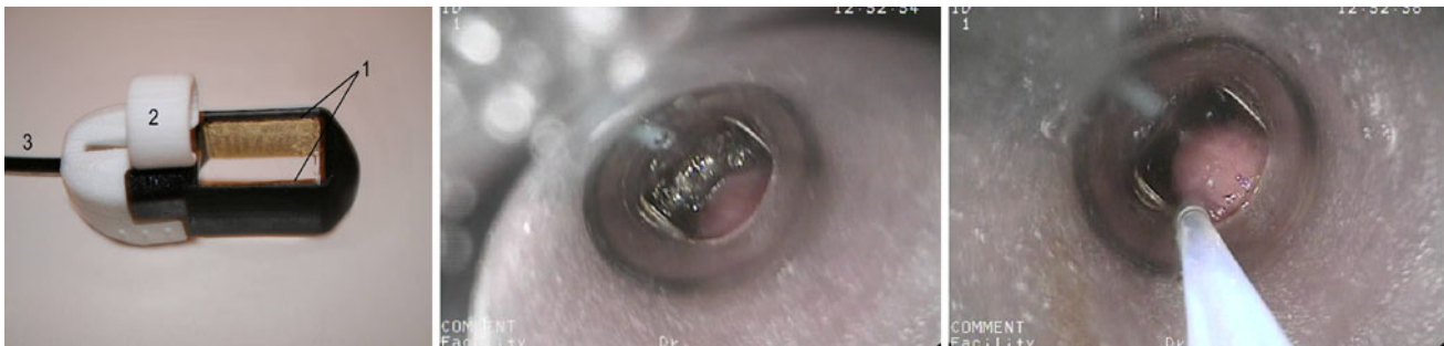
Fig. 3 Image of an EndoVE prototype ( left ) that is then attached to the endoscope head: 1 the electrodes, 2 holder for attachment to the head of an endoscope, 3 cable connection. Middle and right view through the endoscope head of esophageal tissue being drawn into the device chamber. On the right the tissue under pressure has entered the
