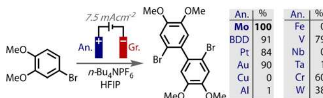
Figure 14. Surface modification through in situ generation of active Mo V coating on anode.
