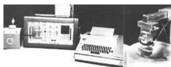
Fig. 3 Automatic particle size analyzer for AgBr particles as designed by Holland and Feinerman. 28
