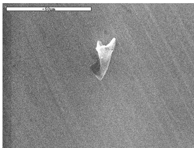
Fig. 4 SEM image of a Ni-graphene coating. Sample 3. Graphene particle in nickel coating
