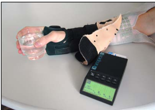
Fig. 12. Prototype of a multi-channel textile neuroprosthesis: Multi-layer structure comprises electrodes placed for finger and wrist articulation.
