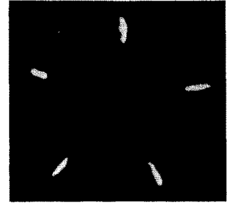
FIG. 12. Suspension of five positively charged particles viewed in the r-\theta plane. V_{ac}=500 v rms, 2V_{dc}=0 , \Omega=210 cy/sec, and \omega_z=23.1 cy/sec. The charge to mass ratio of a single particle was later found to be e/m=0.00765 coulomb/kg.
