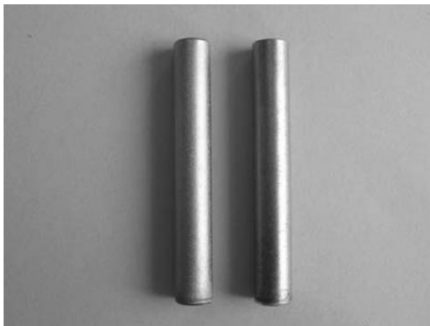
5 Examples of hard chromium deposits on XC38 steel (left) and 304 stainless steel (right) (typical thickness: 25–30 \mu\text{m} ): two samples were coated under same conditions at constant potential in \text{CrCl}_3 \cdot (\text{H}_2\text{O}) \text{ChCl} based eutectic liquid
