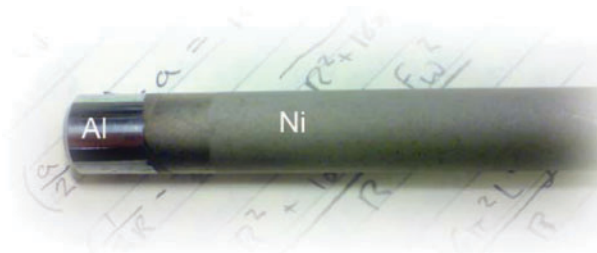
9 10 mm diameter Al rod coated with electroless (immersion) Cu from IL solution and then adherent electrolytic Ni (10 \mu\text{m} ) from conventional aqueous Watts Ni bath
