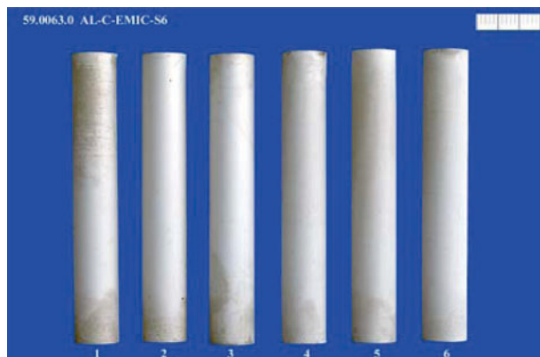
3 Aluminium deposition on mild steel under different pre-treatment regimes: samples shown were electroplated under identical conditions but initial chemical pretreatment was varied to facilitate adhesion tests; all samples show even, homogeneous Al deposit
