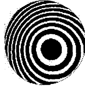
Figure 7a. The masking layout for \theta_{scan} = 15^\circ , \phi_{scan} = -45^\circ , F = 9 cm, n = 5 .
