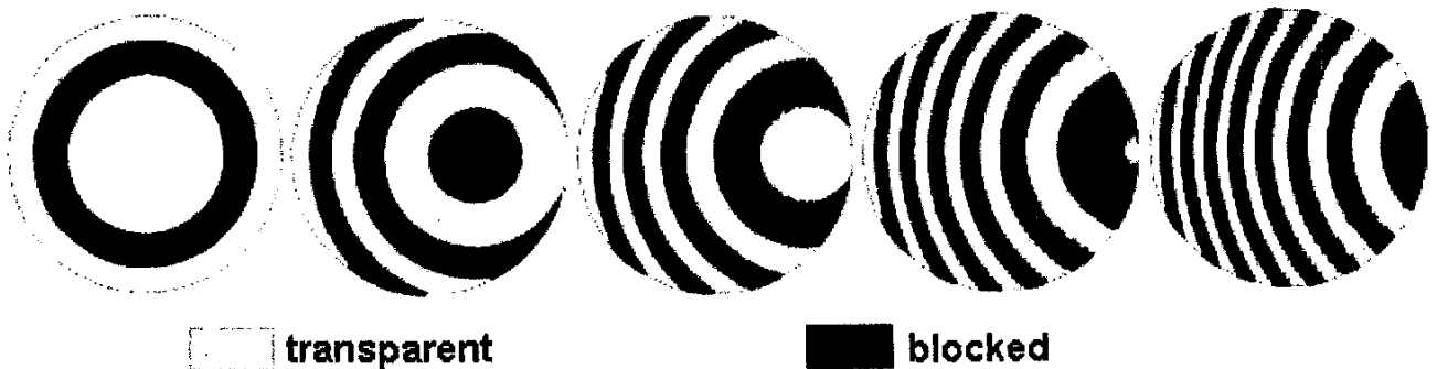
Figure 5b. The masking of the wafer for a diameter of D = 20 cm and a focal length of F = 40 cm.
