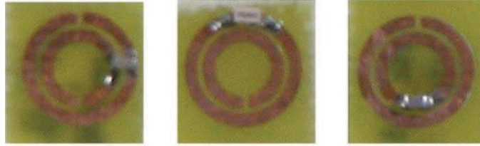
Figure 3.9: SRR devices with capacitors mounted post-fabrication [11]
