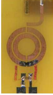
Figure 3.10: Variable-capacitor-diode mounted on an SRR device [82]
