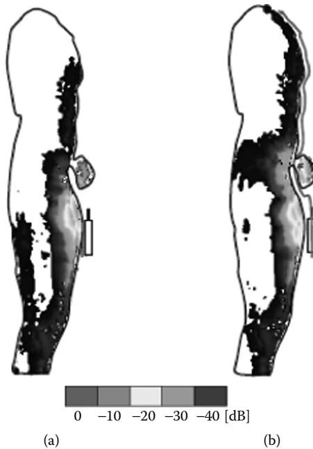
FIGURE 5.21 Qualitative comparison of the unaveraged SAR distribution in the user's body for (a) cellular phone-only and (b) cellular phone with hands-free cases (0 dB = 4.5 W/kg). (From Troulis, S. E., W. G. Scanlon, and N. E. Evans. 2003. Phys Med Biol , 48, 84. With permission.)
