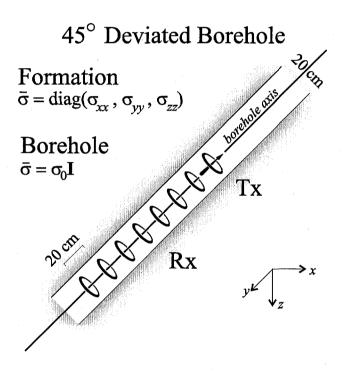
Figure 5. Schematic representation of a deviated borehole in an anistopic formation. The 45° deviation is constrained to the xz-plane. The transmitter (Tx) and receiver array (Rx) are coaxial loops centered on the borehole axis and each separated by 0.2m. Borehole conductivity is  $\sigma_0 = 10$ S/m. Anisotropic formation conductivities are  $\sigma_{xx} = \sigma_{yy} = 1.0$ S/m and  $\sigma_{zz} = 0.25$  S/m.
