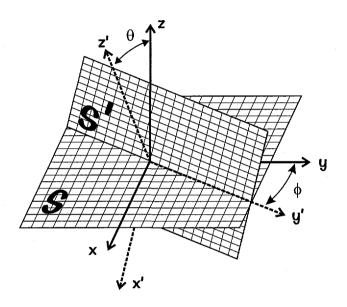
Figure 3. Geometric relationship between the model reference frame (x, y, z) and the principal axes reference frame (x', y', z'). The plane labeled S intersects the origin and is perpendicular to the z axis. The plane labeled S', representing the bedding planes, intersects the origin and is perpendicular to the z' axis. Angles  $\phi$  and  $\theta$  represent the 'strike' and 'dip' of the plane S' with respect to the plane S.
