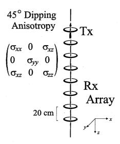
Figure 7. Schematic representation of two models constructed for an internal consistency check of the FD solution. Shown are the receiver (Rx) coil spacing, FD reference frame and formation conductivity tensor for each of the two models. The conductivity tensor of the formation is given by equation (11) where  $\sigma_{\perp} = 0.1$ S/m and 1.0S/m. The transmitter (Tx) frequency is 100kHz.
