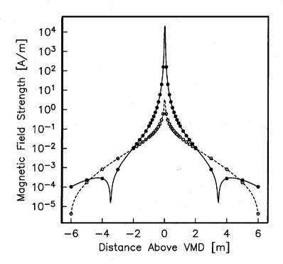
Figure 4. Comparison of analytic (lines) and FD (symbols) of the axial magnetic field magnitude due to a 100 kHz vertical magnetic dipole embedded in an anisotropic wholespace. Vertical and horizontal conductivities of the wholespace are 0.1 and 1.0 S/m, respectively. Open symbols and dashed lines represent the imaginary component of the field while closed symbols and solid lines represent the real component.
