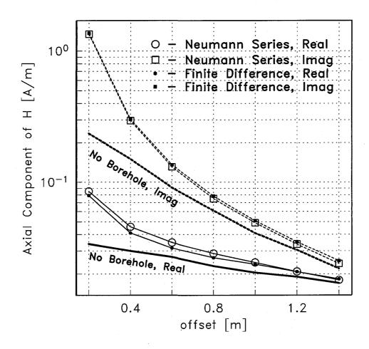
Figure 6. Comparison of the magnetic field along the axis of a 45° dipping borehole due to an axially aligned 160 kHz magnetic dipole. Shown here is the difference between the total field and the field due to the same source located in vacuum.
