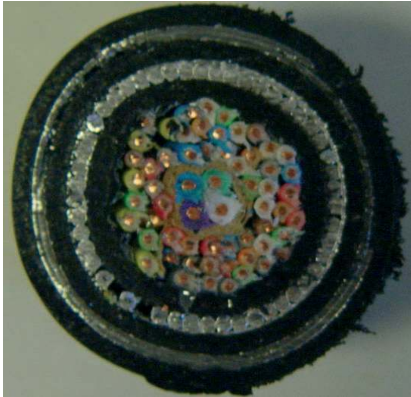
Figure 1.7: Telecommunication cable used in Banverket systems
