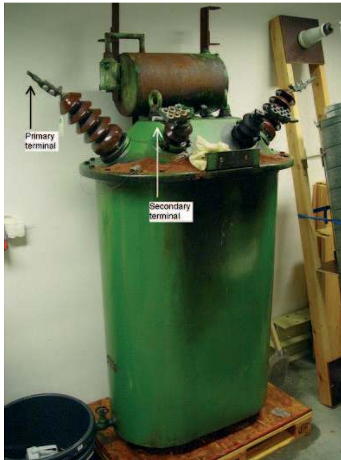
Figure 1.8: Typical booster transformer used in the Banverket systems
