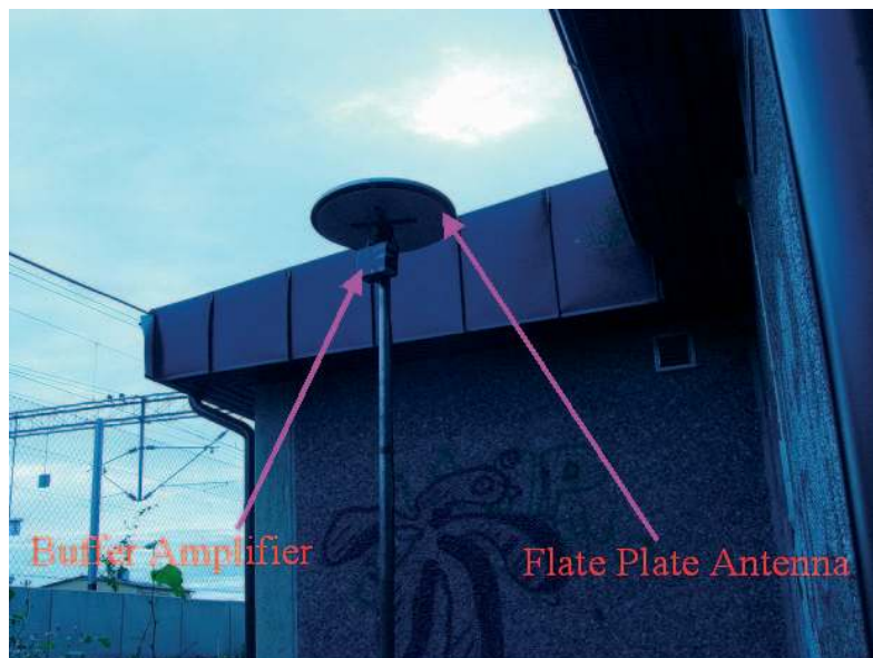
Figure 6.3: Vertical electric field measuring system for lightning
