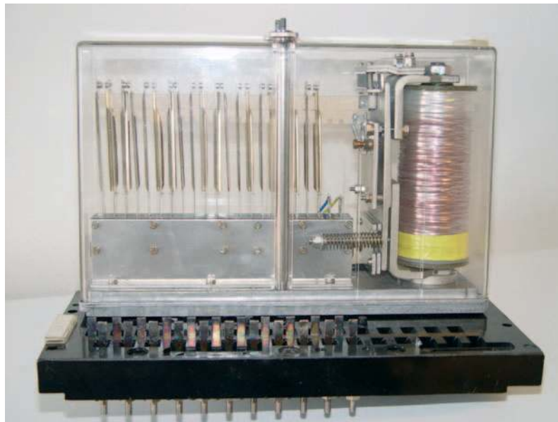
Figure 1.10: Typical relay unit used in the track circuits
