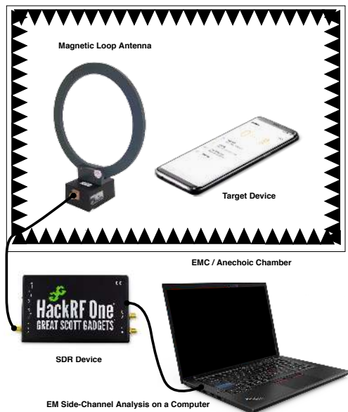
Figure 3: An illustration of how an EM side-channel analysis would be performed in a forensic investigative setting. Target device is placed inside an EMC/Anechoic chamber and observed using an SDR device that is connected to an EM analysis software framework.
