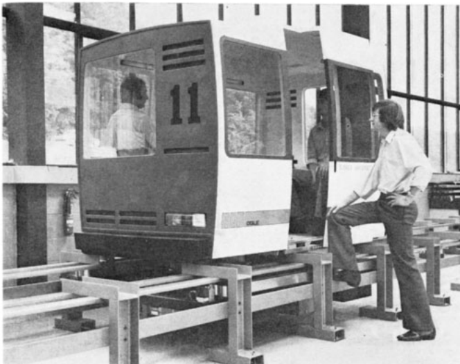
Figure 6. University of Sussex 1 ton 4 passenger vehicle using controlled DC electromagnets for suspension.
