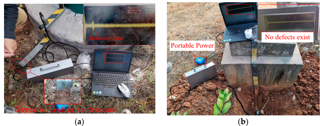
Figure 15. (a) Grounding lead wire inspection of 35 kV steel pipe tower and (b) detection of grounding flat steel of 220 kV transmission tower.
