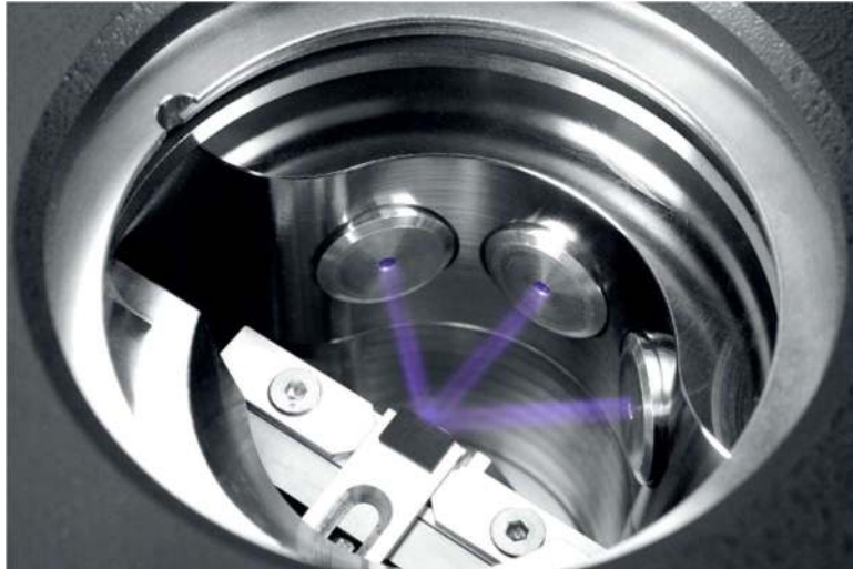
Figure 2.3 Leica TIC 3x sample chamber with triple argon ion beams. Sample location is at beam convergence point.
