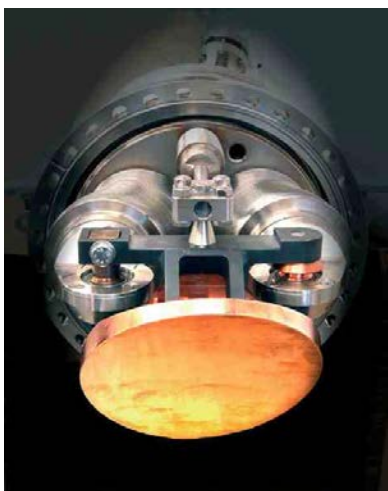
Figure 3: Picture of the launching mirror of the TEXTOR ECRH system. The focusing mirror and the push and pull rods for actuation of horizontal and vertical rotation are visible.
