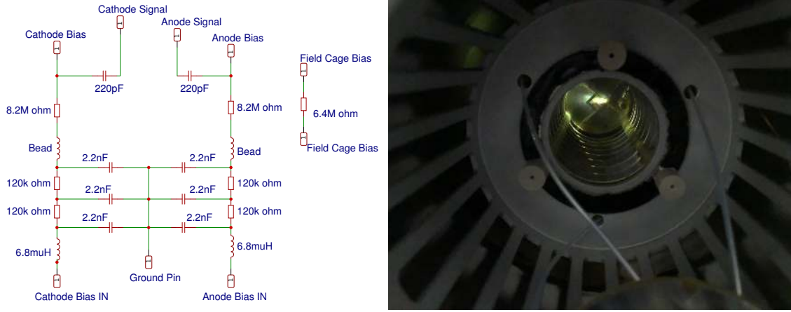
Figure 4. Left: Schematic of the electron drift circuit; Right; view into drift region from the collection plane upward. Light is being shone through the UV transmitting fiber and illuminating the gold photo-cathode.
