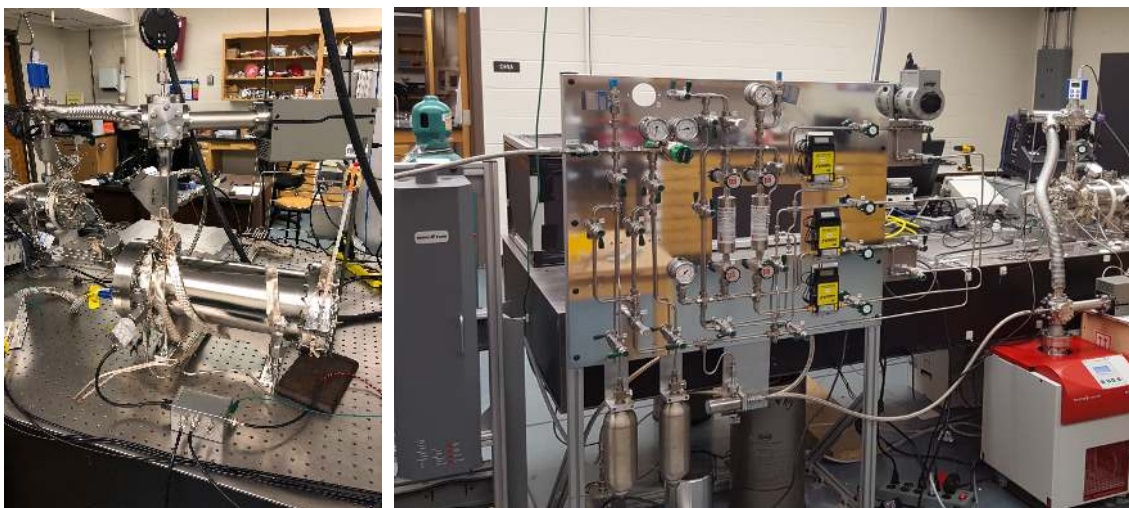
Figure 2. Left: Photograph of the 5 litre pressure vessel with the electron drift apparatus inside. Right: Photograph of the gas system that supports this vessel and another similar one, used as a holding volume for gas in this study.
