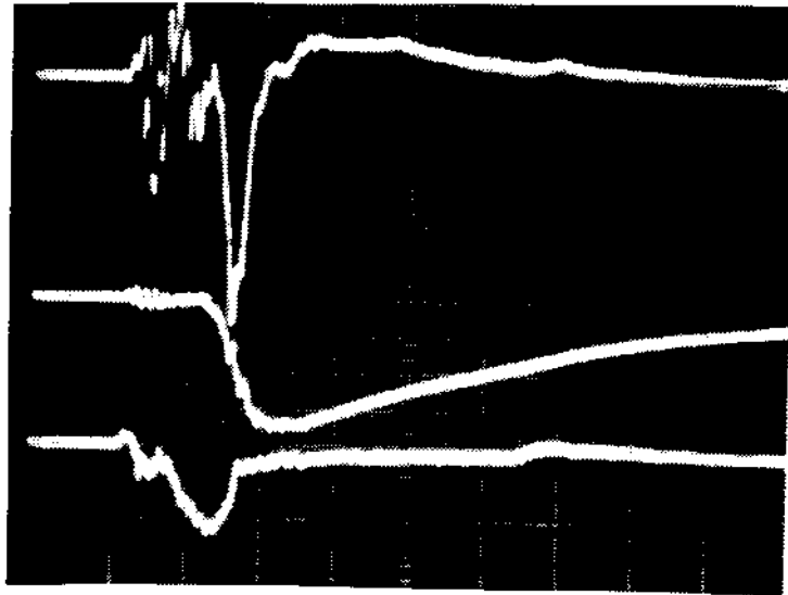
Figure 6: Typical waveforms of emitted current (upper trace, 2 \text{ A/cm}^2 per small division (sd), 100 \text{ ns/sd} ), charge (middle, 200 \text{ nC/sd} ), and switching voltage (lower trace, 1 \text{ kV/sd} ) obtained from a ceramic PLZT sample without extraction voltage.
