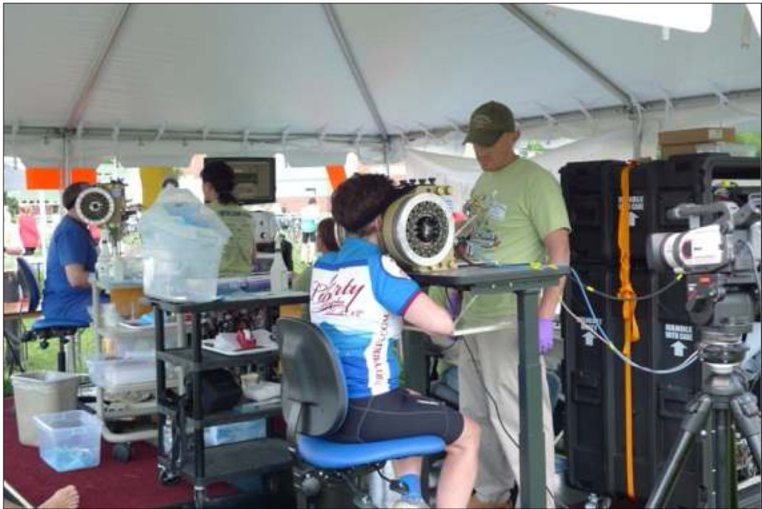
Fig. 2. The prototype EPR tooth dosimetry systems have been operated successfully in field conditions, including measurements of walk-up volunteers at a local cancer fundraiser. Measurements were performed within a tent and a truck using power supplied by a remote generator.
