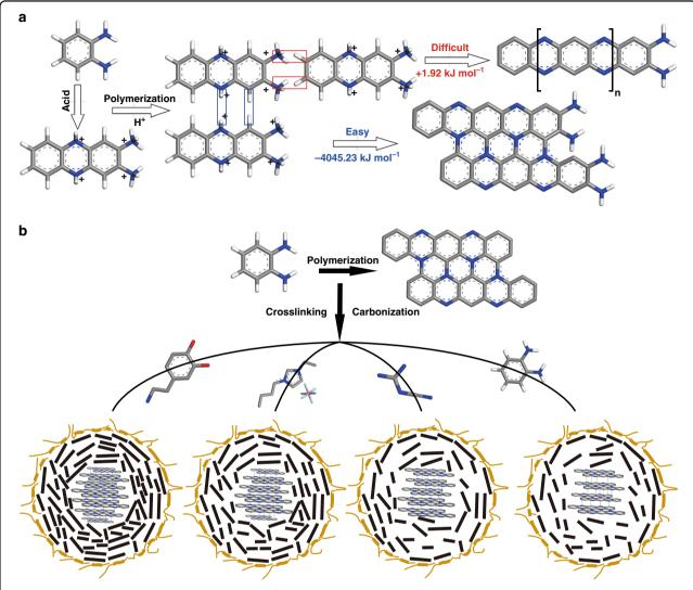
**Fig. 6 Formation process and structural analysis of CDs. a** Formation energies of longitudinal and transverse growth of CDs from oPD. **b** Core–shell structures formed by four kinds of CDs
