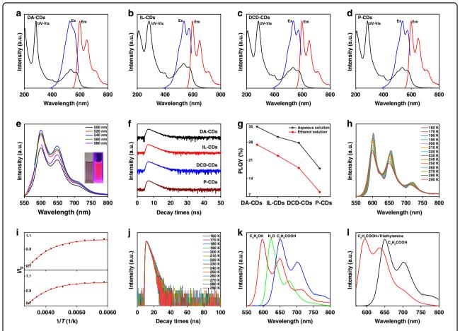
Fig. 2 Spectral characterization of CDs. a–d Em, Ex, and UV-Vis spectra of four CDs in ethanol. e Excitation-dependent spectra of P-CDs. f PL dynamics of the four selected samples. g QYs in aqueous and ethanol solutions. h, i Variable temperature PL spectra and j normalized PL dynamics of P-CDs. k, I Fluorescence emission spectra of P-CDs in different solvent environments
